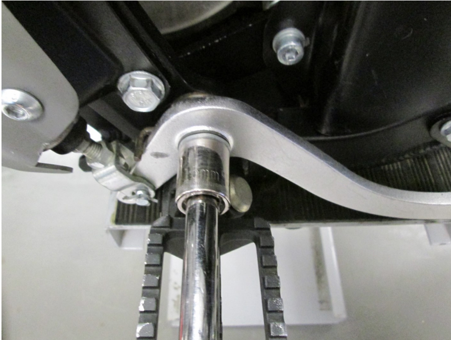
3) Remove brake pedal with 15mm socket.
