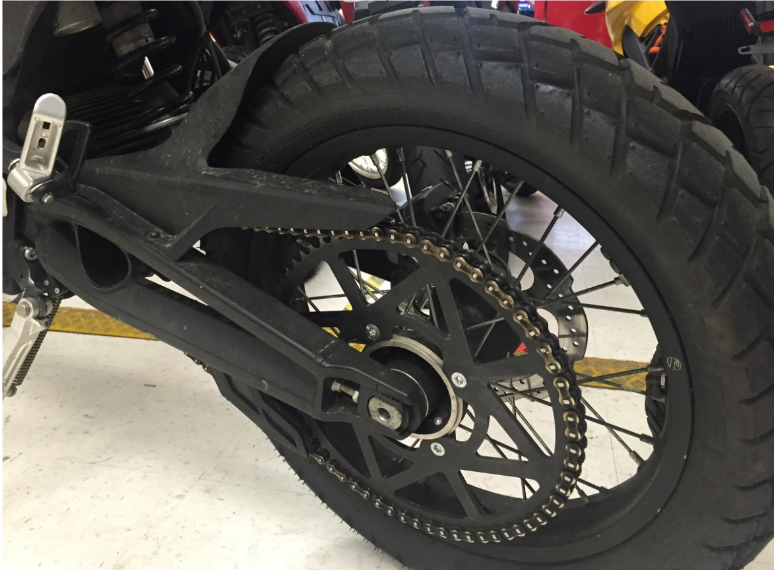
Completed chain assembly
